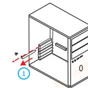
1. Use a screwdriver to remove the bezel and screws on the main unit
