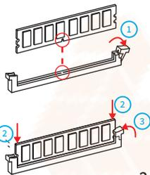
1. Pull the clips on both ends of the memory slot outward, and the memory strip corresponds to the protruding position of the slot to determine the direction of installation
