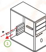
1. Use a screwdriver to remove the bezel and screws on the main unit
