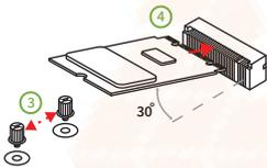
3. Tighten the screw base screwed into the length M.2 module to the M.2 interface distance hole
