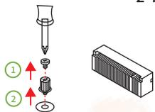
1. Remove the screw from the screw base
