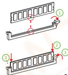
1. Pull the clips on both ends of the memory slot outward, and the memory strip corresponds to the protruding position of the slot to determine the direction of installation
