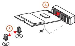
3. Tighten the screw base screwed into the length M.2 module to the M.2 interface distance hole
